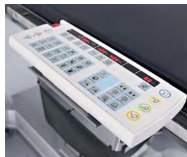
Remote user interface for control of all relevant C-arm functions from within the sterile field
